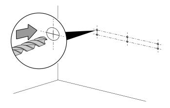
3. Insert appropriate wall plugs into the bore holes depending on the type of wall. Position the holder on the wall as shown and attach the holder in place with the 6 screws.
