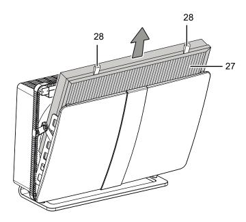
3. Clean the HEPA carbon filter (27) with a dry, lint-free cloth if it is slightly dirty. If heavily soiled, dispose of the HEPA carbon filter (27) in accordance with the national regulations and remove the new HEPA carbon filter from the plastic cover.
