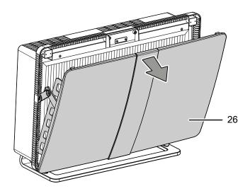
2. Pull the strips (28) to take the HEPA carbon filter (27) out of the device.
