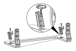
2. Correctly screw the large feet to the designated points on the back of the device.
