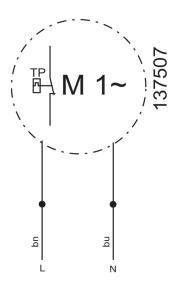
During operation, electric motors heat up. Under certain circumstances (excessively high ambient or fluid temperatures, heavy contamination, etc.), the motor temperature may exceed the safety limit of the electrically isolated parts. In order to avoid engine damage, various types of temperature monitoring are possible, of which at least one must be installed on site. (Exception: fans with thermal contacts integrated in the motor current)
