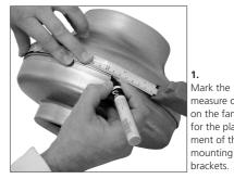
1. Mark the measure of **B** on the fan for the placement of the
