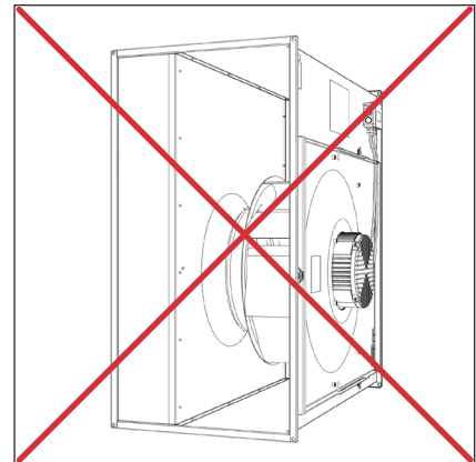
Motor bracket facing to the side.
