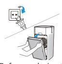
Before replacing the filter, please stop this appliance and cut off power.
