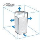
When the appliance is working, it must be placed on a dry, flat and stable floor, with at least 30cm space reserved around it.
