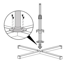
4. Push the stand's protective cap (7) onto the screwed connection.
