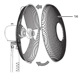
2. Make sure that the two parts are fixed by all fastening clips (15).
