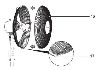
2. Make sure that the two parts are fixed by all four fastening clips (17).
