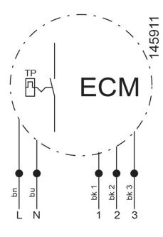
In case of step speed control the desired step 1, 2 or 3 must be switched to the phase L.
