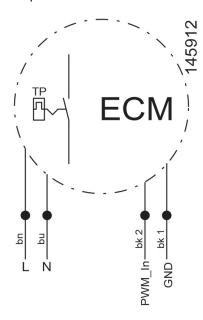
In case of stepless speed control via PWM, a PWM signal with a frequency of 1-5kHz and an amplitude of 5-10V must be applied to the input PWM\_In.
