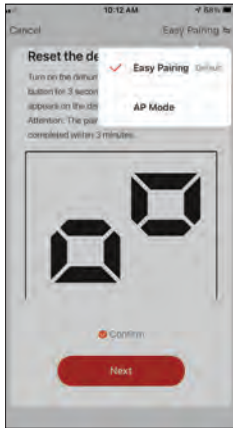
Step 4: Tap on "Easy Pairing" on the top right and select "AP Mode".
