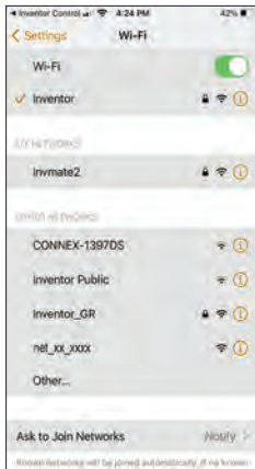
Step 7: From your mobile device settings, connect to the dehumidifier's network "net_xx_xxxx". Return to the app and press "Next".
