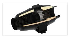
Due to the conic impeller and special blade profiling the circumferential air speed increases thus providing higher air pressure and capacity as compared to standard axial fans. The diffuser, the specially profiled impeller and the directing vanes at outlet from the fan casing distribute air flow in such a way as to attain the best combination of high performance and high pressure at low noise level. The fan casing is equipped with an airtight terminal box for connection to power mains.
